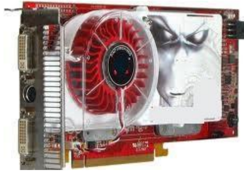
Picture 2. 15: GPU and Fan System
