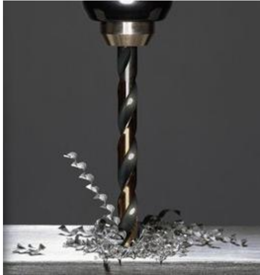
Picture 1.16: Drilling process
