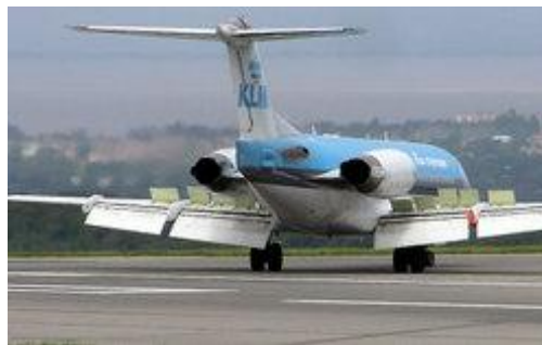
Figure 2.7 showing position of flap and airbrake/spoiler flight controls
