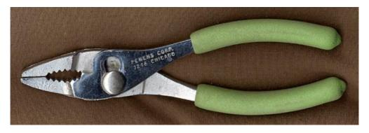
Figure 3.12: Slip joint pliers
