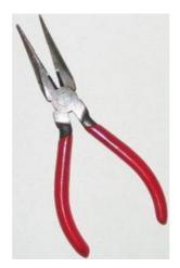
Figure 3.13: Needle nose pliers
