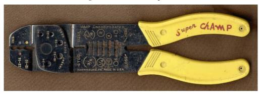
Figure 3.15: Electrical wire stripping and terminal crimping pliers
