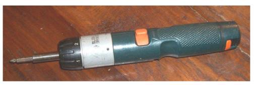
Figure 3.8: A rechargeable battery-powered electric screwdriver.
