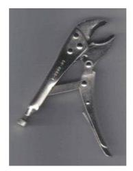
Figure 3.17: Lock jaw pliers, also called vise grip or "mole grips".
