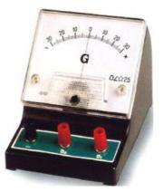
Figure 6.5: A galvanometer
